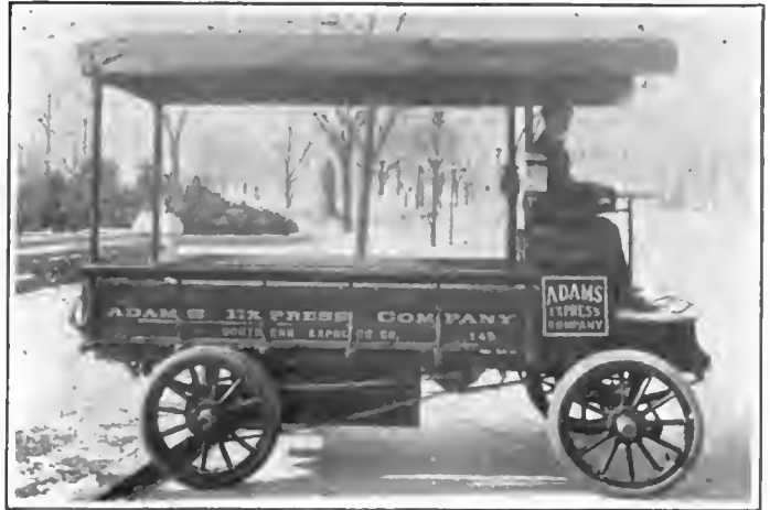
LANSDEN CHAIN-DRIVEN ELECTRIC EXPRESS WAGON.
